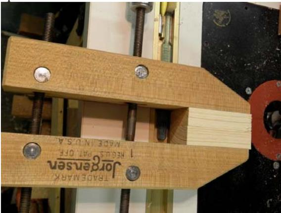
Or by moving the jaws close but then closing only the near screw, you can apply pressure at the very tips of the clamps:
