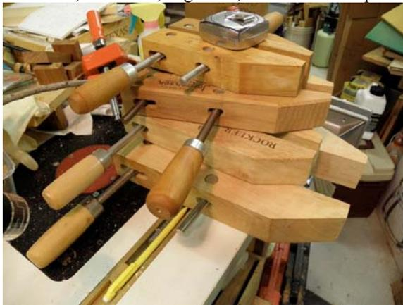
The length is an indication of the length of the wooden member, what I call the body size, others call the jaw size. Typically the jaws open to about half the stated body size. And the reach (depth) is also
