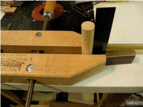
A really nice thing about the flat bodies is that you can actually clamp the clamp to a workbench to hold your work still or more stable (for example when using the drill press), or for edge planing. Here I've used
