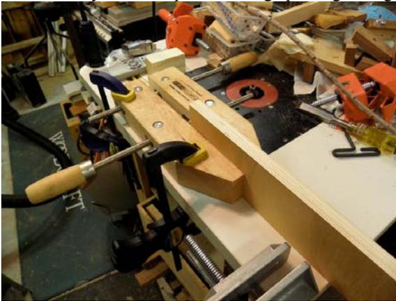
And Here's how to hold a (narrow) plank for surface planing or surface work:
