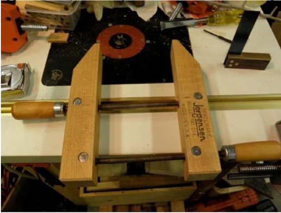
The inserts can rotate a bit due to slots cut around the screws, here's how much they can typically turn (maybe 15-20 degrees?):
