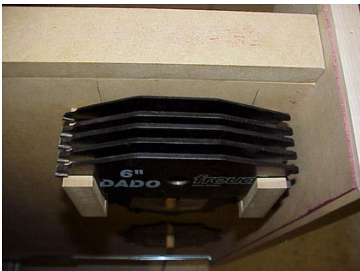
**Figure Six: Blade Caddy—Chipper Holder**
