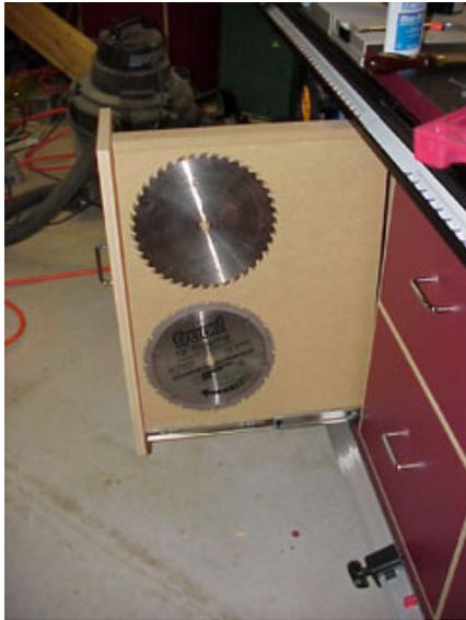
**Figure Four: Blade Caddy—Blade Side**
