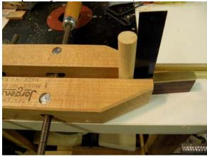
A really nice thing about the flat bodies is that you can actually clamp the clamp to a workbench to hold your work still or more stable (for example when using the drill press), or for edge planing. Here I've used
