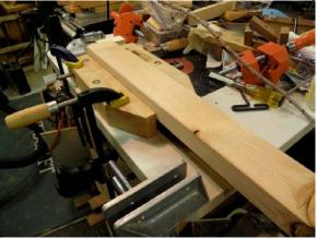
Special Trick: unfortunately the screws don't have a quick release feature allowing you to change the opening by large amounts except by turning the screws. Here's a way to make many turns quickly while keeping the jaws relative to each other. Hold them on opposite sides and crank them like a bicycle,
