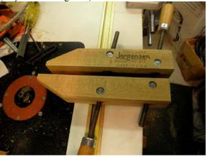
By closing them together then you can apply pressure distributed all along a joint which is good for glue-ups:
