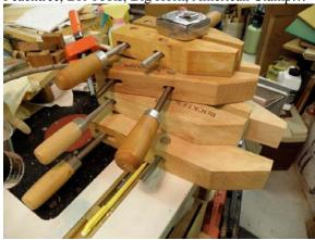
The length is an indication of the length of the wooden member, what I call the body size, others call the jaw size. Typically the jaws open to about half the stated body size. And the reach (depth) is also
