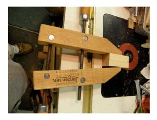
Notice how the wood bodies lie flat – this can be very useful for holding small items to be routed - Clamp the item tightly with the item and the two bodies flat on the table and hold the clamp, keeping your fingers well clear:
