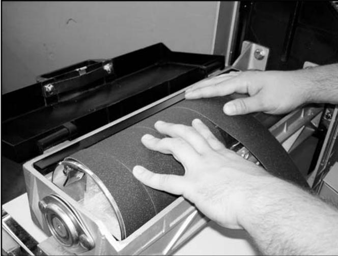
3. Once you have completely wrapped the drum, keep tension on the strip and insert the remaining end of the strip into the slot in the drum.
