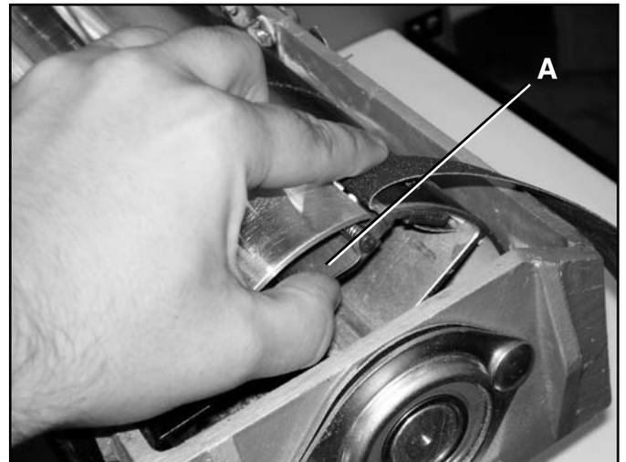
2. Stand in front of the unit and roll the drum away from you as you wrap the abrasive strip around the drum. Make sure not to overlap the strip or to leave any gaps in between the strip and drum. **SEE FIG 4B.**
