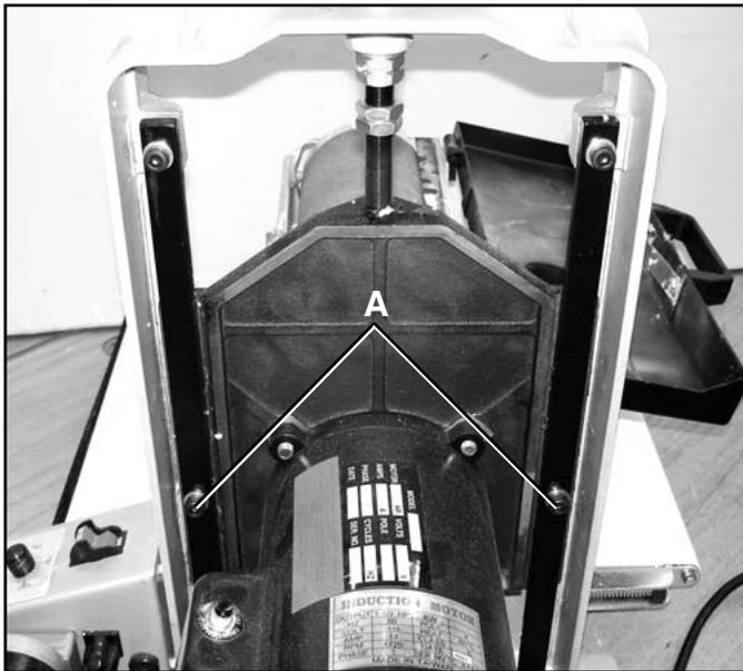
2. Loosen or tighten each screw as required. Make adjustment in 1/4 turn increments until the desired fit is achieved.
